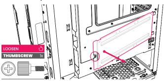
Loosen the thumb screw on the SSD backplate to remove it, for easy installation of the 2.5" SSD's.
