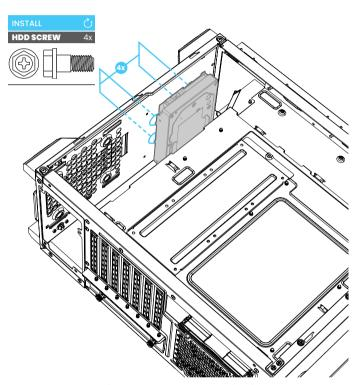
Hold the 3.5" HDD into place and secure it with 4x HDD screws from the bottom.
