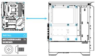
Install the ATX motherboard using 9x motherboard screws. For M-ATX Motherboards follow the motherboard instructions to move the stand-offs to the correct position.
