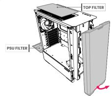
Remove front panel by pulling the panel from below.
