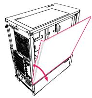
Remove the glass panel, set it aside in a safe location to prevent damage.
