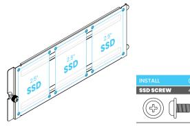
The backplate can hold up to 3x 2.5" SSD's. Use 4x SSD screws per SSD to secure it in location.
