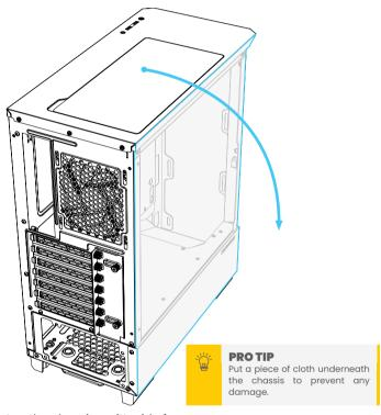
Lay the chassis on it's side for easy access.
