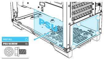
Slide in the power supply from the side and secure it with the 4x PSU screws. It is recommended to connect all needed cables beforehand.
